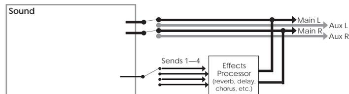
Effects parameters are edited separately from either the Program or the Mix, using Effects Edit Mode (more in Chapter 6). In Program Edit Mode, each of the four sounds in the Program has its own Effect Level control and can be assigned to any one of the four effect buses. Effects settings, Effect Level and Bus information are saved with the Program when you store it back into memory.
