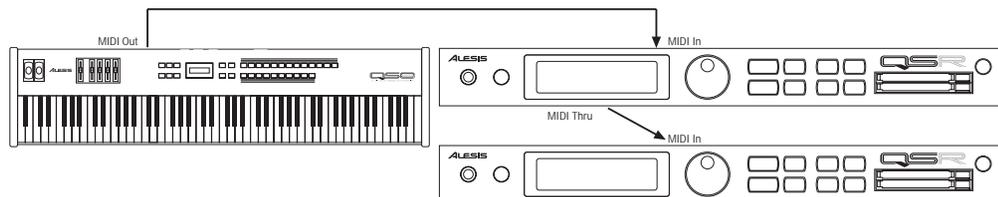
The QSR’s [MIDI OUT] connector sends *System Exclusive* data (see the MIDI supplement) to a storage device for later recall, or to another QSR. When the [MIDI OUT] connector’s mode is switched to “Thru” (Global Edit mode, page 12), it can function as a second [MIDI THRU] connector and resend MIDI data received on the [MIDI IN] from the controller to other MIDI devices.
