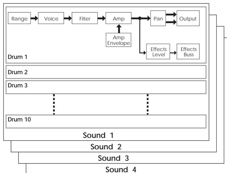
When Drum Mode is enabled, the sound will have fewer parameters for editing. Consequently, not all Function buttons will respond when pressed as when Drum Mode is turned off. Specifically, the LFOs and all Envelopes (with the exception of the Amp Envelope) are unavailable. In addition, the parameters in most other functions will differ. See page 82 for more information about Drum Mode.
