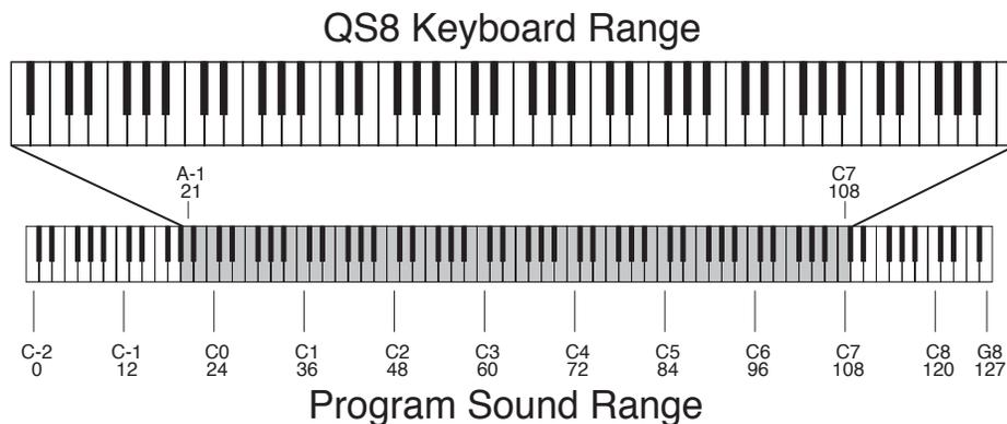
**TIP:** By setting the lower limit above the high limit, you can create a “hole in the middle” effect. This makes the sound appear to have two zones. All notes from the bottom of the keyboard to the high limit note will play, and all notes from the lower limit to the top of the keyboard will play, but the notes between the high limit and the lower limit will not play. This can be further enhanced in Mix Mode by using the Range function in Mix Edit Mode to cap-off the lower and high limits.
