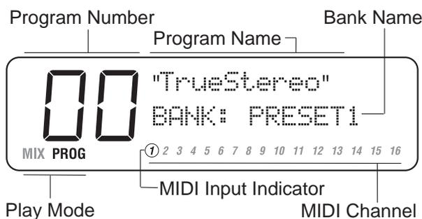
The current mode (PROG) is displayed in the bottom-left corner. The current Program number (00) is directly above. To its right can be found the Program's name (TrueStereo) and the currently selected Bank name (PRESET1). The current MIDI channel appears below the Bank name.
