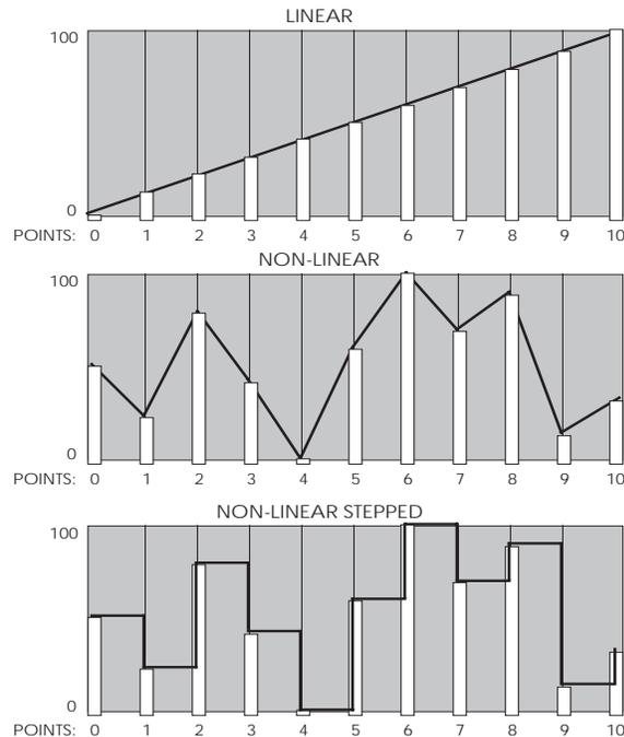
**TIP:** The Tracking Generator can be used to turn a variable control, such as the Mod Wheel or velocity, into a switch by setting all of the points to 0 except for point 10. Only near the maximum input will anything other than 0 come out of the Tracking generator. You can patch the Mod Wheel somewhere else in addition to the Tracking Generator, giving you gradual control of one function with the full range of the Mod Wheel, while switching on a second function only at the top of the wheel.
