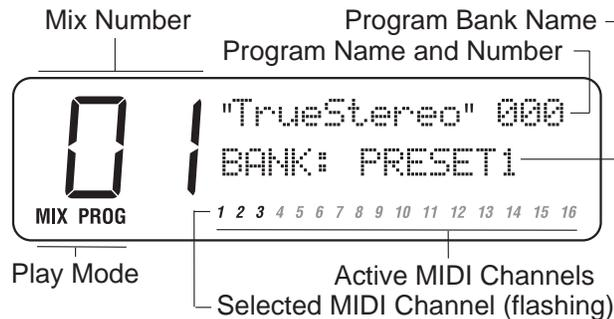
The [ ◀ MIDI ▶ ] buttons are used to select one of the 16 channels in the Mix. The actual channel number will be whatever channel was last selected. In the illustration above, channel 1 is shown flashing. If the channel 1 number in your display is not flashing, Use the [ ◀ MIDI ▶ ] buttons to select channel 1.
