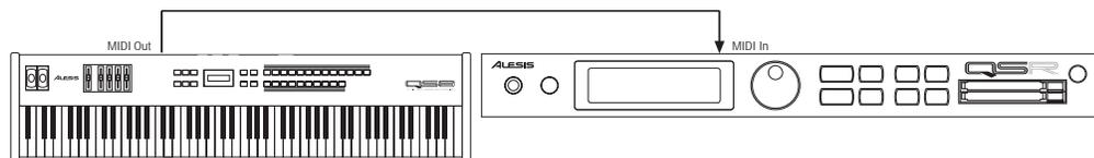
If you are using the QSR in the middle of the MIDI chain (example: as the second unit of a three device chain), connect the QSR’s [MIDI THRU] to the third device’s MIDI IN connector in order to route the first device’s MIDI out information to the third device.
