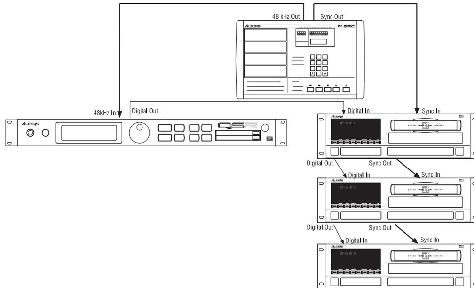
*Tip:* With this type of connection, the ADAT tracks will remain in tune with the QSR even when the BRC's pitch value is adjusted.
