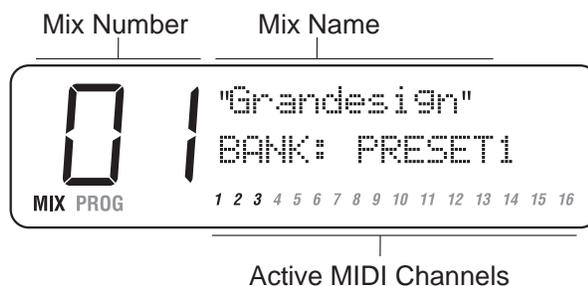
The current mode (MIX) is displayed in the bottom-left corner. The current Mix number (01) is directly above. To its right can be found the Mix's name (Grandesign) and the currently selected Bank name (PRESET1). The Active MIDI Channels (1, 2 and 3) are shown at the bottom. In a Mix that uses all 16 MIDI channels (such as the Mixes found in the General MIDI Bank), the display would light up all 16 MIDI channel indicators.
